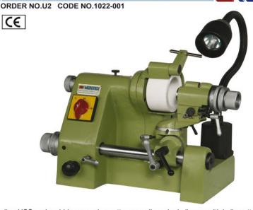
For grinding HSS and carbide engraving cutter as well as single lip or multiple lip cutters of various shapes such as radiused cutters or negative taper angle of cutters. The universal index head is provided at 24 positions so that any particular angle or shape can be obtained, free 3600 or 100 rotation is allowed for grinding End Mills, Twist Drill, Lathe Tools, only replace the attachment to the index head without any complex setup.
