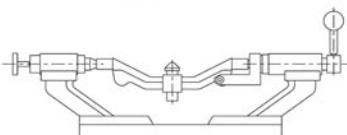
The dresser can be dressing any concave and convex of grinding wheel
