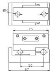
This fine precision-made unit dresses grinding wheels to any angle from 0°-60° degrees with new smoothness and accuracy.
