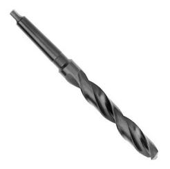
HSS TMX TAPER SHANK GENERAL PURPOSE DRILLS, 118° POINT, BLACK OXIDE, 1-1/16" DIAMETER X 6-5/8" FLUTE LENGTH X 11-1/4" OVERALL LENGTH (OAL) WITH # 3 MORSE TAPER SHANK
