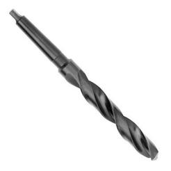
HSS TMX TAPER SHANK GENERAL PURPOSE DRILLS, 118° POINT, BLACK OXIDE, 1-7/64" DIAMETER X 7-1/8" FLUTE LENGTH X 11-3/4" OVERALL LENGTH (OAL) WITH # 3 MORSE TAPER SHANK
