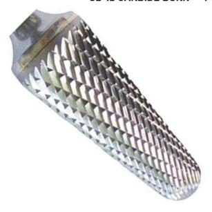
TAPER SHAPE 8° INCLUDED ANGLE WITH RADIUS END - DOUBLE CUT: 1/8" CUT DIAMETER X 1/8" SHANK DIAMETER X 1/2" LENGTH OF CUT X 1-1/2" OAL, **INCLUDED ANGLE 8°**
