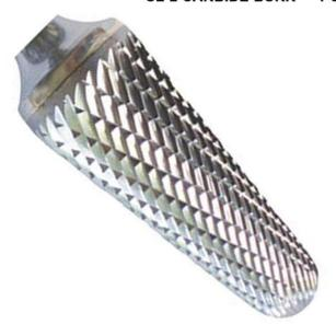
TAPER SHAPE 14° INCLUDED ANGLE WITH RADIUS END - DOUBLE CUT: 5/16" CUT DIAMETER X 1/4" SHANK DIAMETER X 7/8" LENGTH OF CUT X 2-5/8" OAL, **INCLUDED ANGLE 14°**
