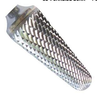
TAPER SHAPE 14° INCLUDED ANGLE WITH RADIUS END - DOUBLE CUT: 1/2" CUT DIAMETER X 1/4" SHANK DIAMETER X 1-1/8" LENGTH OF CUT X 2-7/8" OAL. **INCLUDED ANGLE 14°**
