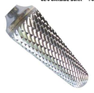
TAPER SHAPE 14° INCLUDED ANGLE WITH RADIUS END - DOUBLE CUT: 5/8" CUT DIAMETER X 1/4" SHANK DIAMETER X 1-5/16" LENGTH OF CUT X 2-15/16" OAL. **INCLUDED ANGLE 14°**
