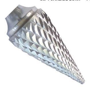
POINTED CONE SHAPE 14° INCLUDED ANGLE - DOUBLE CUT: 3/8" CUT DIAMETER X 1/4" SHANK DIAMETER X 7/8" LENGTH OF CUT X 2-1/2" OAL, **INCLUDED ANGLE 14°**
